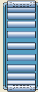
Sheet steel cage of the radial bearing
