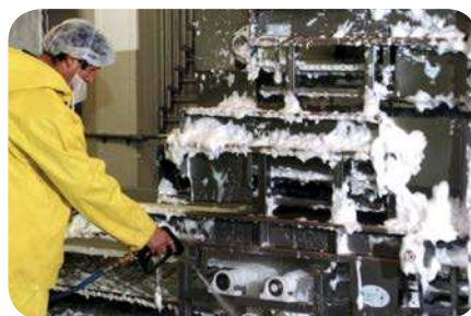
High pressure washdowns can deflect and open seals, contaminating and washing out the lubricating grease
