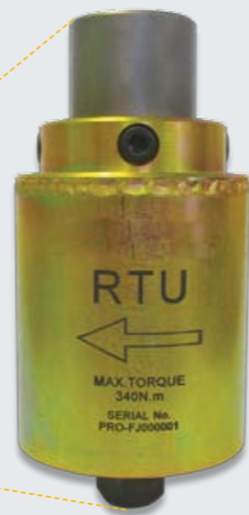
Modification of RTU for Track Bolt Tightening
